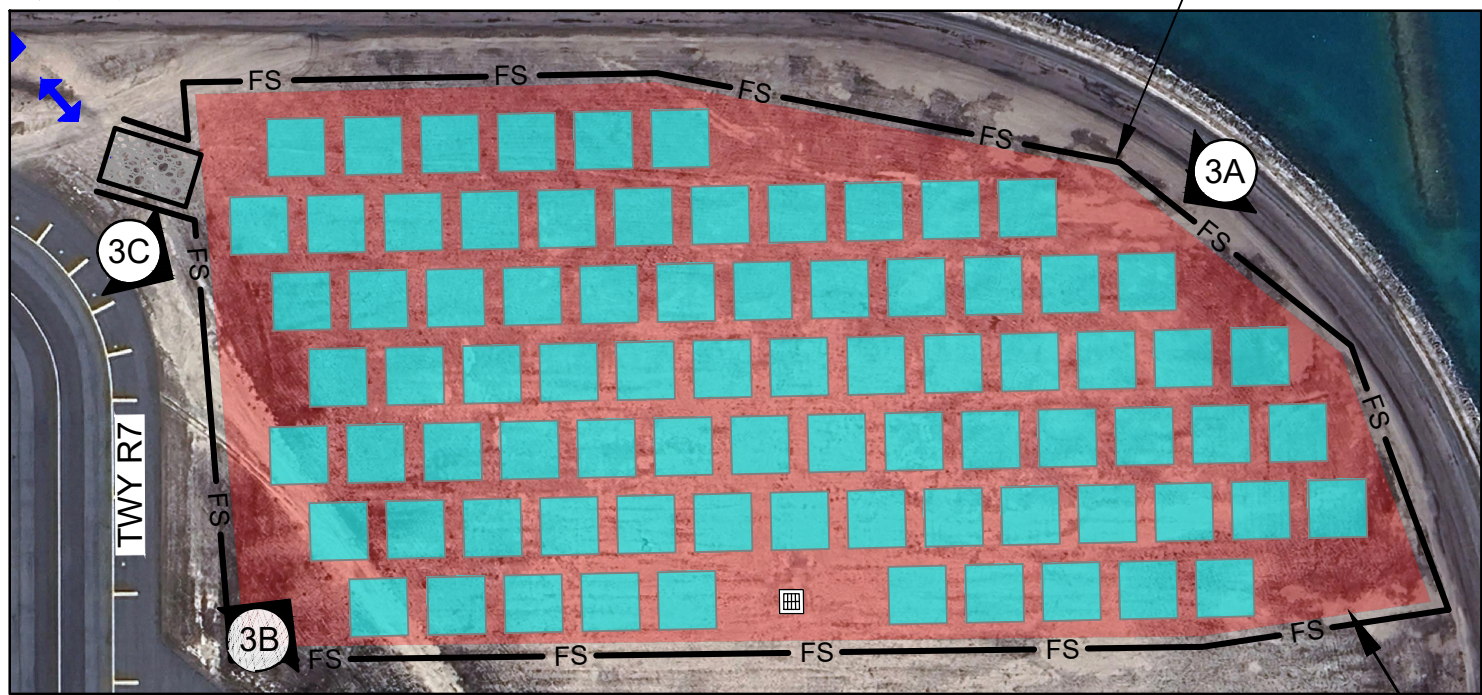
IMPROVEMENT PLAN FOR STOCKPILING AREA 3 SCALE: 1" = 200' AREA: ~ 14.2 ACRES APPROXIMATE CAPACITY: ~ 80 STOCKPILES, ~ 32,000 CY
